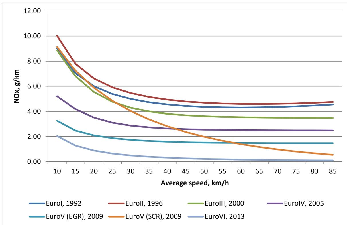
**Figure 3** Effect of speed on NOx emissions from a small HGV
